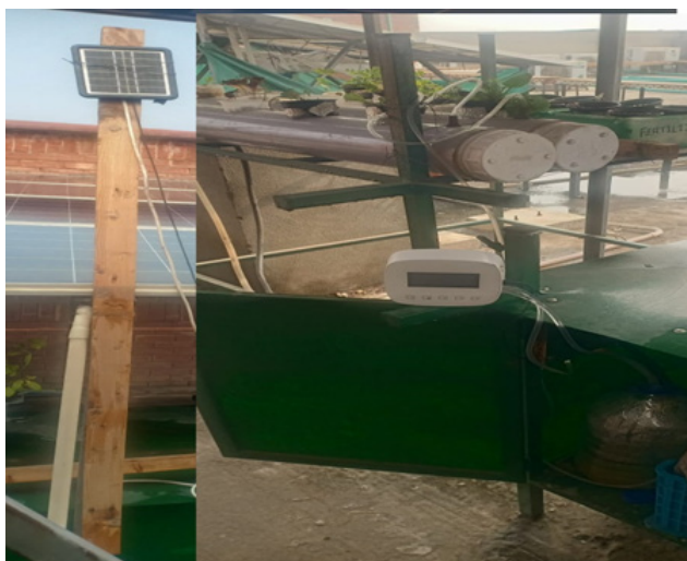
The solar light-based automatic nutrient pump
