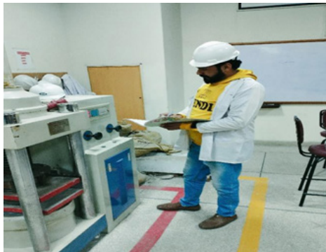
Figure. 4: Compression test of fly ash bricks
