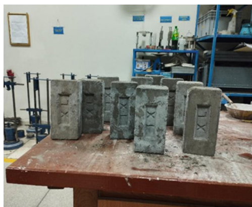
Figure. Efflorescence visible on samples
