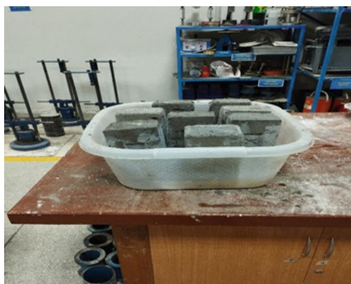
Figure.6: Efflorescence test of fly ash bricks
