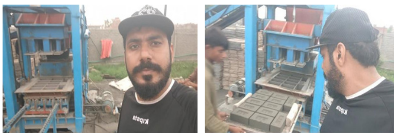
Figure.3 (c) Placing the mixture into dies (d) Demolding of the bricks
